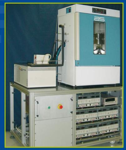
The system has been designed to satisfy the needs of Industry Research Centres requiring the development and the testing of Gas Sensor Heads.
