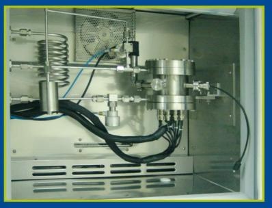
A volumetric mixture is prepared via massflow controllers starting from pure gases. Different full scale massflow controllers are used to obtain the required precision over the concentration mixture range.
