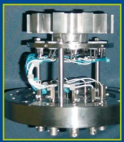
The test cell can accept up to 10 sensor heads and has a volume of 1/2 lt.
